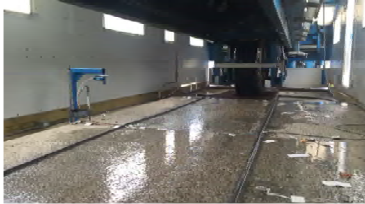
Figure 40: Heavy Vehicle Simulator Water Saturated Test
